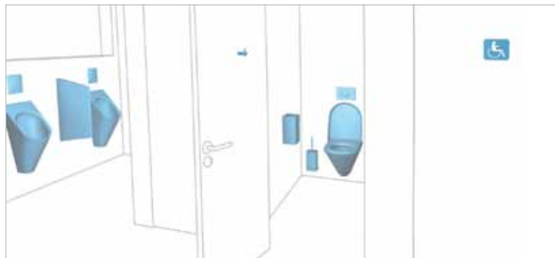
TOILET CABINES/URINAL CABINES: urinals, urinal divider, urinal flush valves, hook, toilet roll holder, toilet brush and brush holder, toilet with seat, flush plate
